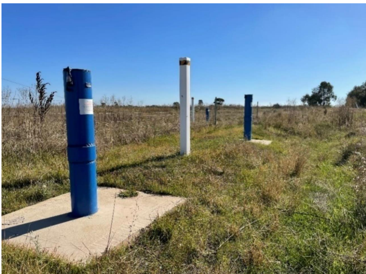
Figure 9 Nested State Observation Bore site in the West Campaspe GMA showing bores that monitor different aquifer layers.
